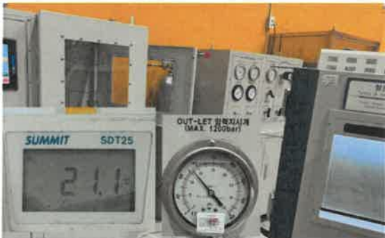
Test Pressure : 455 Bar, Temperature : 21.1℃, Cycle Test : 50 Cycle
