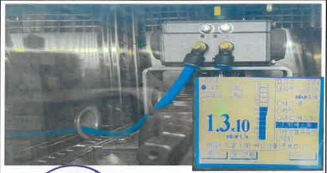
Leakage Stem Seal: 1.3 E-06
