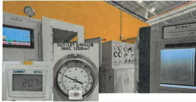
Test Pressure : 378 Bar, Temperature : 20.7°C
