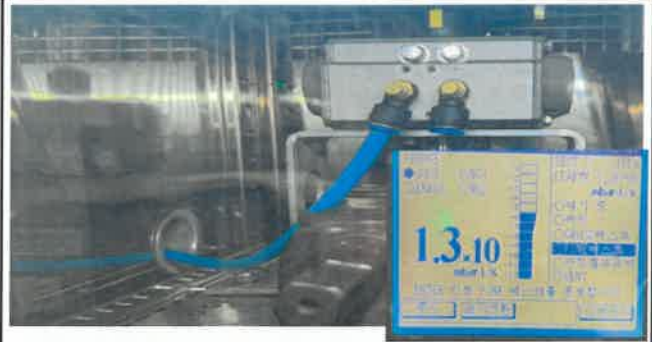
Leakage Stem Seal: 1.3 E-06
