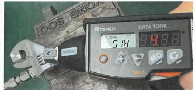
Operating Torque(N.m): Open: 4, Close: N/A
