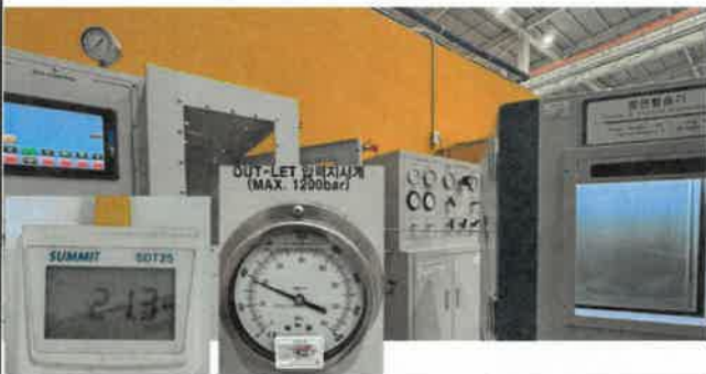
Test Pressure : 378 Bar, Temperature : 21.3°C, Cycle Test : 50 Cycle
